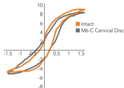
The Load-Displacement Curves of the M6-C closely approximate intact controls.
