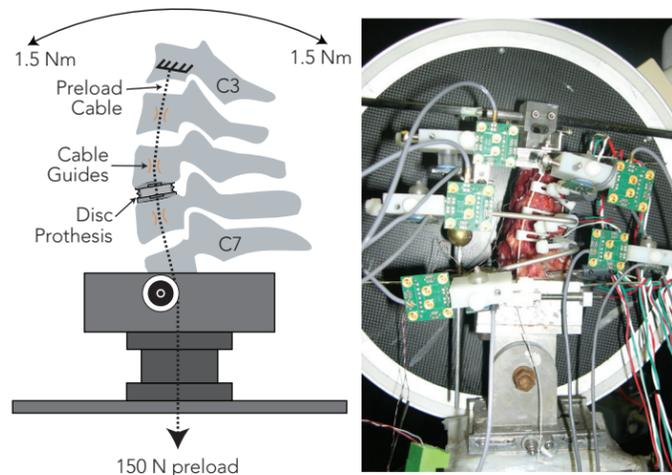
Schematic of a cervical spine mounted in the biomechanical test set-up (left). A 150N follower load is applied through the center of rotation of each segment via the Preload Cable. A moment of  $\pm 1.5$  Nm is applied and the resulting ROM is measured with the attached sensors (right).
