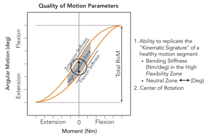
Kinematic Signature C5-C6 Flexion-Extension Load-Displacement Curves
