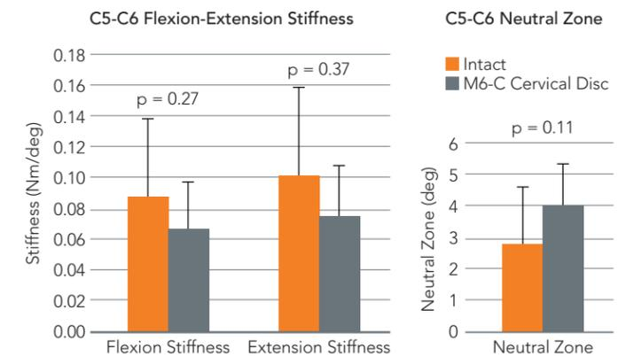
No difference in flexion/extension stiffness in the high flexibility zone or in the magnitude of the neutral zone between intact segments and implanted M6-C.
